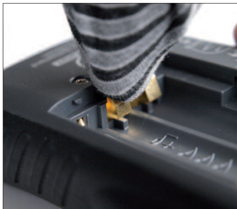
Photo 12: A battery contact is getting cleaned.
