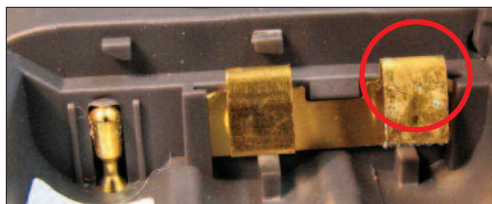
Photos 8 Battery contacts with clear signs of leaked batteries.
