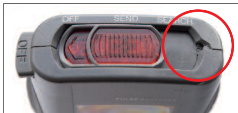
Photo 3 Case damaged at the top right corner. Such devices must be checked by an official Barryvox service center and not be used any longer!
