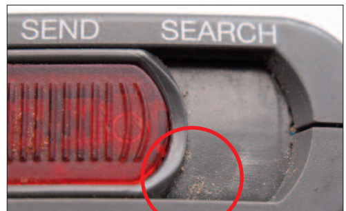
Photo 1 A contaminated main switch
