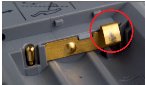
Photo 9: A contaminated lower battery contact
