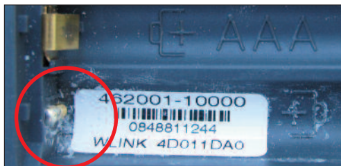
Photo 15: A contaminated main battery connector
