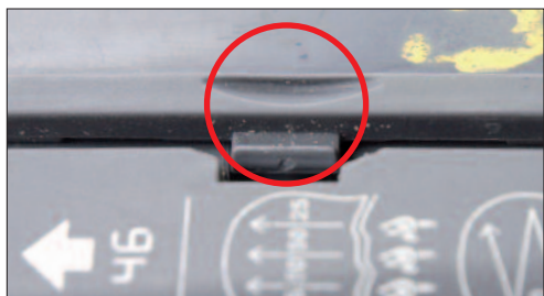
Photo 6 The destruction is caused by users who have tried to open the battery case with an inappropriate tool and by pushing directly on the locking hook. Such damage is not covered by warranty.
