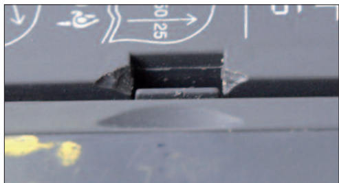
Photo 5 If the battery compartment is damaged, the cover may not lock properly anymore.
